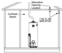
All Air From Outdoors - Using A Single Permanent Opening FIGURE 8B.
